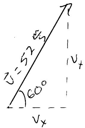
a)  $\vec{V}_f = 52 \frac{\text{m}}{\text{s}} \cdot \sin 60^\circ = \boxed{45 \frac{\text{m}}{\text{s}}}$
